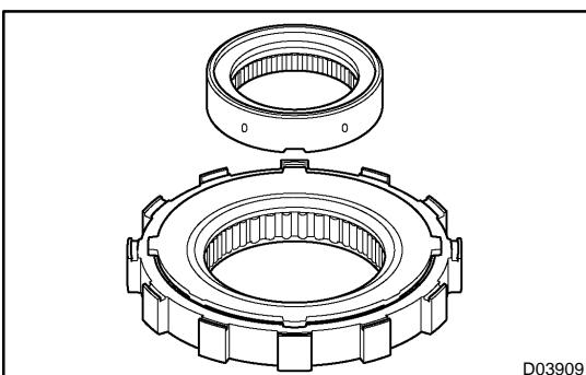
(b) Remove the inner race from the one-way clutch No.1.
