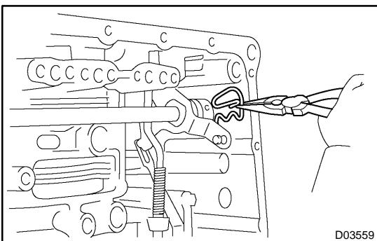
**15. REMOVE MANUAL VALVE LEVER SHAFT**
