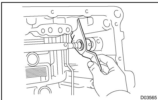
(f) Remove the manual valve lever shaft and the manual valve lever.
