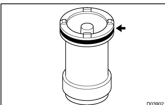
(c) Remove the O-ring from the piston.
