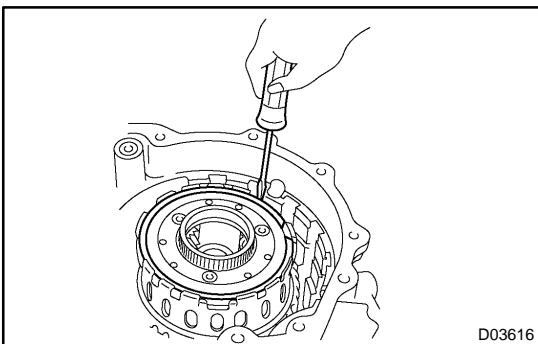
**36. REMOVE REAR PLANETARY GEAR**
