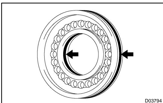
(b) Remove the 2 O-rings from the U/D brake piston.
