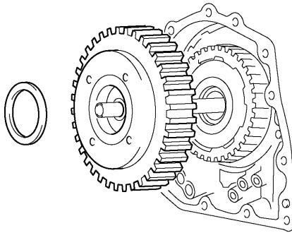
**31. REMOVE DIRECT CLUTCH ASSEMBLY**
