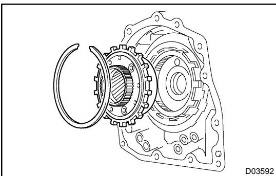
(b) Remove the rear planetary gear from the transaxle case.
