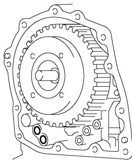
**30. REMOVE TRANSAXLE CASE APPLY GASKET**
