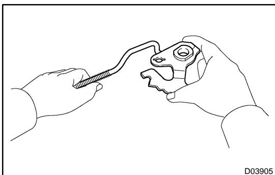
(g) Remove the parking lock rod from the manual valve lever shaft.
