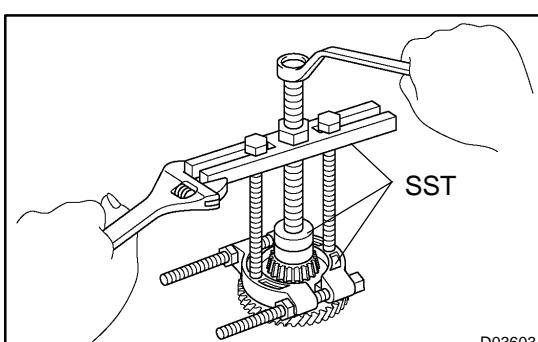
(c) Using SST, remove the tapered roller bearing RH.
