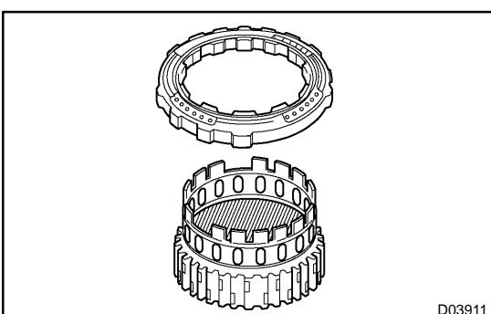
(b) Remove the brake hub from the 2nd brake cylinder assembly.
