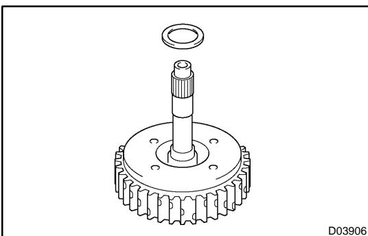
(b) Remove the thrust bearing from the forward clutch.
