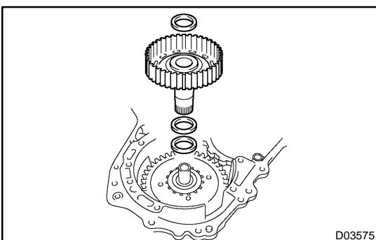
(c) Remove the multiple clutch hub, 2 thrust bearing and bearing race from the transaxle case.
