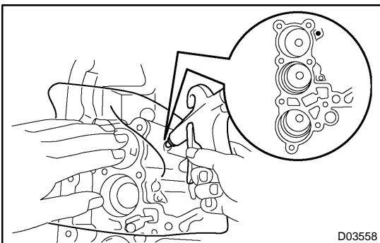
(f) Apply compressed air (392 kPa, 4.0 kgf/cm<sup>2</sup>, 57 psi) to the oil hole and remove the B<sub>3</sub> accumulator piston and 2 springs.
