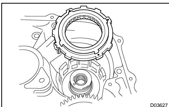
(b) Remove the one-way clutch No.2 from the transaxle case.
