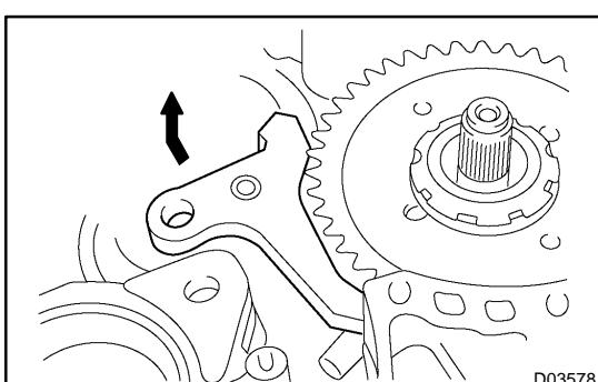
(e) Remove the spring, the pin and the parking lock pawl.
