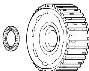
(b) Remove the thrust bearing from the rear planetary sun gear.
