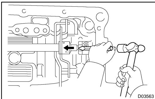
(d) Using a chisel and a hammer, unstake and remove the spacer.
