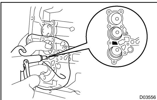
(b) Apply compressed air (392 kPa, 4.0 kgf/cm<sup>2</sup>, 57 psi) to the oil hole and remove the C<sub>3</sub> accumulator piston.
