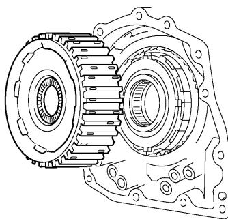
**32. REMOVE REAR PLANETARY SUN GEAR ASSEMBLY**
