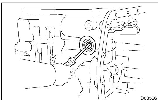
(h) Using a screwdriver, remove the oil seal.
