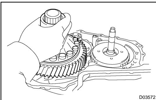
**21. REMOVE DIFFERENTIAL ASSEMBLY**
