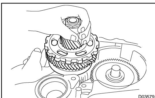
(d) Remove the U/D planetary gear assembly from the transaxle case.
