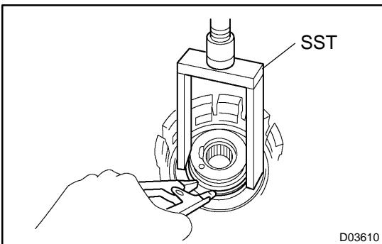
(c) Using SST, a snap ring expander and a press, remove the snap ring and return spring.
