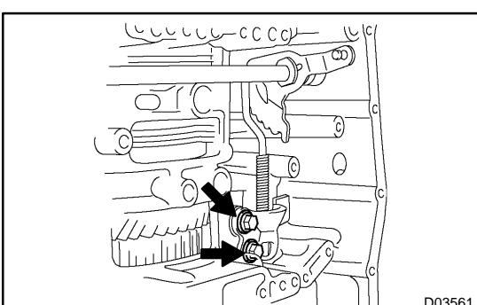
(c) Remove the 2 bolts and the parking lock pawl bracket.
