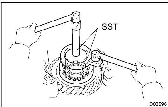
(b) Using SST, remove the nut.
