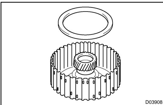
(c) Remove the thrust washer No.1 from the rear planetary sun gear.
