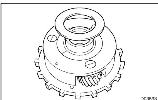
(d) Remove the bearing race from the rear planetary gear.
