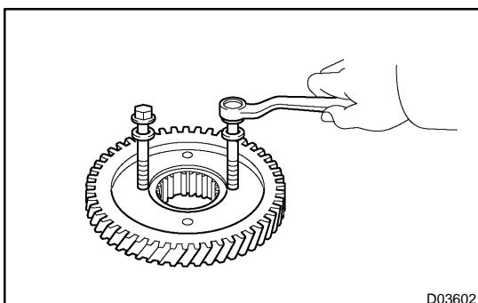
(b) As shown in the illustration, tighten 2 bolts evenly and make clearance of approx. 20.0 mm (0.797 in.) between the counter drive gear and the inner race.
