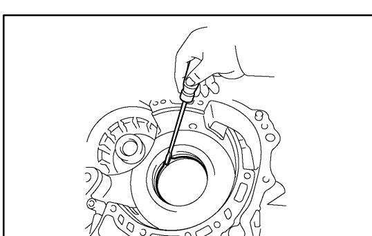
(e) Using a screwdriver, remove the snap ring from the transaxle case.
