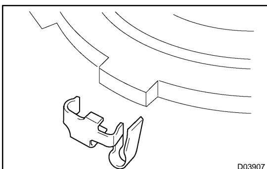
(c) Remove the outer race retainer from the one-way clutch No.2.
