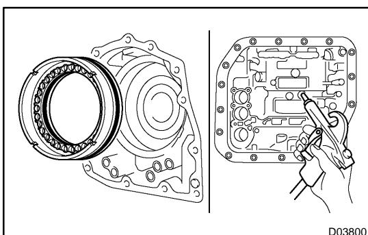
(c) Apply compressed air (392 kPa, 4.0 kgf/cm<sup>2</sup>, 57 psi) to the transaxle case to remove 1st & reverse brake piston.
