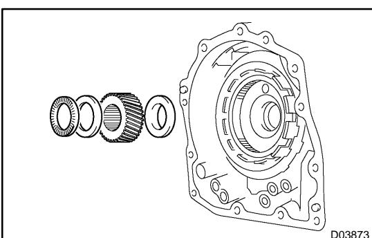
**37. REMOVE FRONT PLANETARY SUN GEAR**
