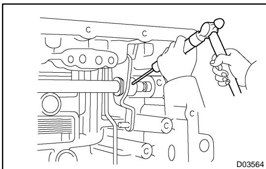
(e) Using a pin punch and a hammer, drive out the pin.
