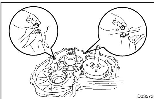
**22. REMOVE 2 APPLY GASKETS**
