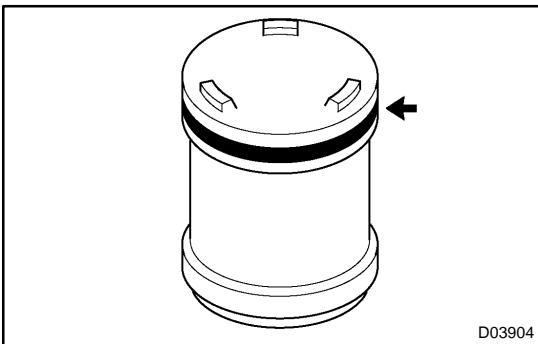
(g) Remove the O-ring from the piston.
