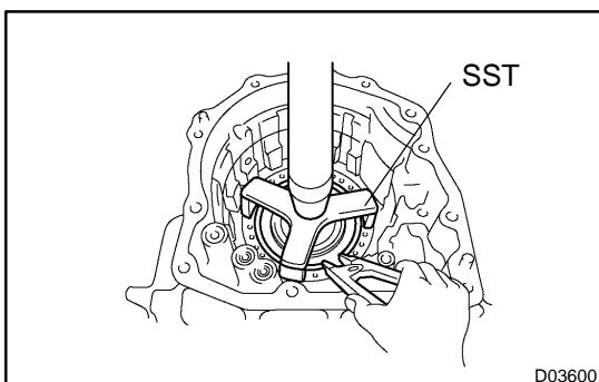
(b) Using SST, a press and a snap ring expander, remove the snap ring and the piston return spring.
