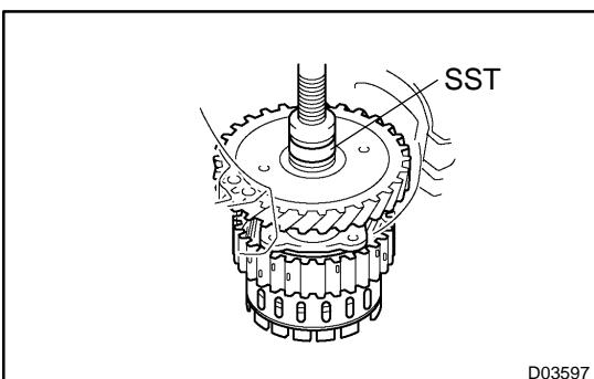
(c) Using SST and a press, remove the front planetary gear assembly from the counter drive gear.
