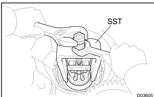
(c) Using SST, remove the needle-roller bearing from the transaxle case.
