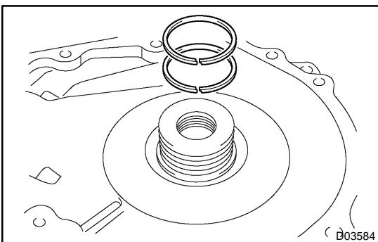
(c) Remove the 2 oil seal rings from the transaxle rear cover.
