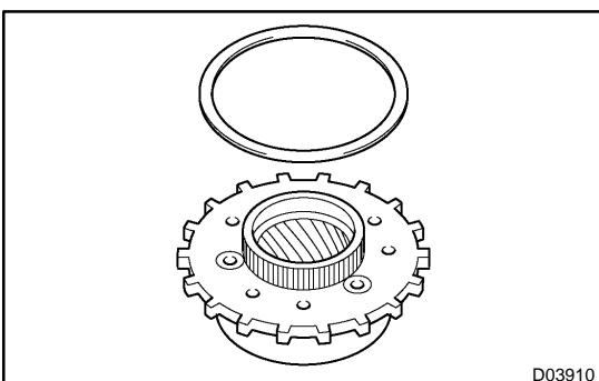
(c) Remove the thrust washer No.2 from the rear planetary gear.
