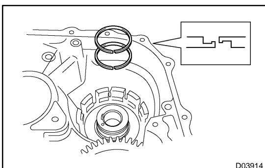
(d) Remove the 2 oil seal rings from the transaxle case.
