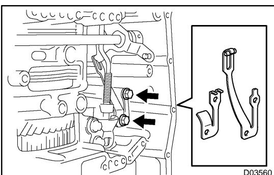
(b) Remove the 2 bolts, the manual detent spring and cover.
