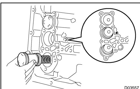
(d) Apply compressed air (392 kPa, 4.0 kgf/cm<sup>2</sup>, 57 psi) to the oil hole and remove the C<sub>1</sub> accumulator piston and spring.
