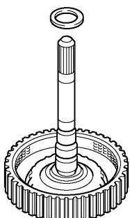
(b) Remove the bearing race from the direct clutch.
